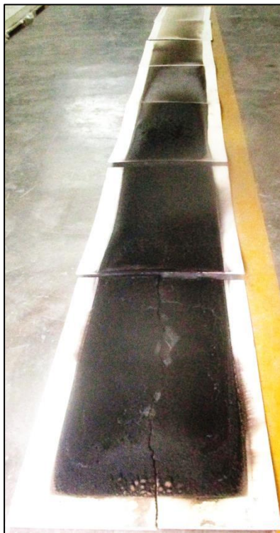
Picture 2 – Specimen located on top of the fire source.
